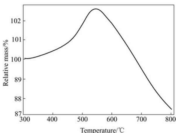
Fig.5 TG curve of 450 °C sample, measured with heating rate of 10 °C/min
