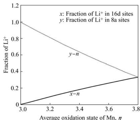
Fig.6 Function of average oxidation state of Mn with fraction of  $\text{Li}^+$  in octahedral 16d sites ( $x-n$ ) and tetrahedral 8a sites ( $y-n$ ) for  $[\text{Li}_{1+y}]_{\text{tet}}[\text{Mn}_{2-x}\text{Li}_x]_{\text{oct}}\text{O}_4$  spinels (Li:Mn=1, at case of  $2x+y=1$ )
