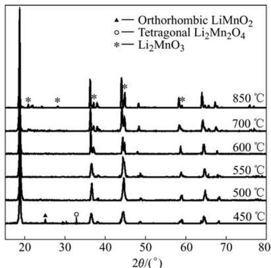
**Fig.3** XRD patterns of Li-Mn-O spinel prepared by sintering precursor at various temperatures for 12 h in air
