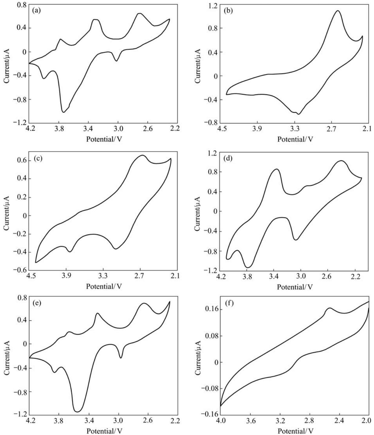
**Fig.4** CV curves of Li-Mn-O spinels prepared by sintering precursor at different temperatures: (a) 450 °C; (b) 500°C; (c) 550 °C; (d) 600 °C; (e) 700 °C; (f) 850 °C
