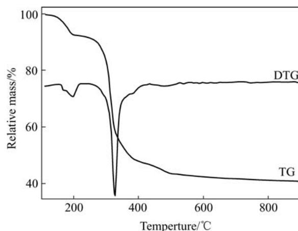
Fig.1 TG-DTG curves of  $\text{LiMn}(\text{C}_2\text{O}_4)(\text{Ac})$  precursor measured with heating rate of  $10\text{ }^\circ\text{C}/\text{min}$
