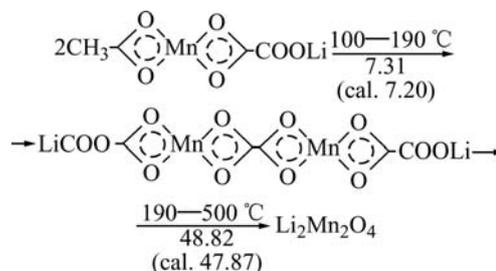
Fig.2 Thermo-decomposition process of  $\text{LiMn}(\text{C}_2\text{O}_4)(\text{Ac})$
