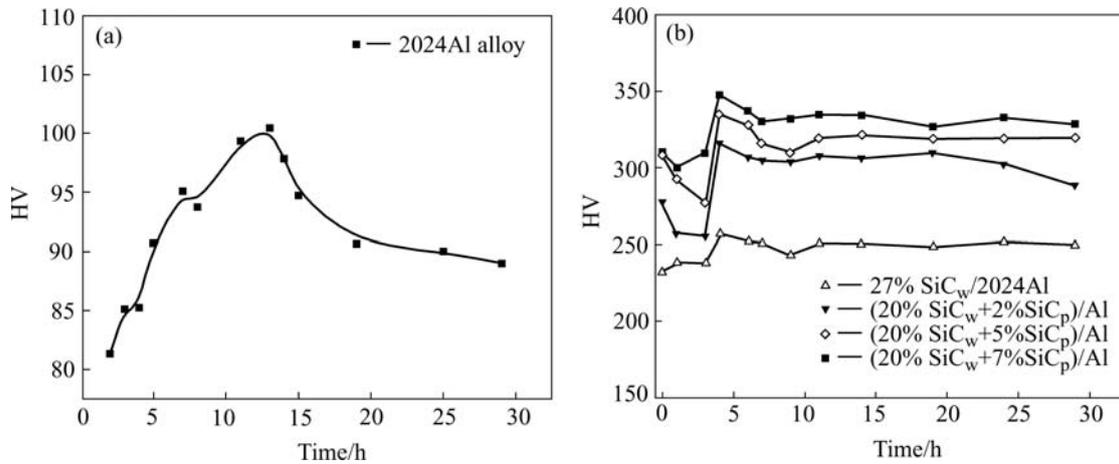
Fig.2 Variation of hardness of 2024Al and composites with time during 190 °C aging
