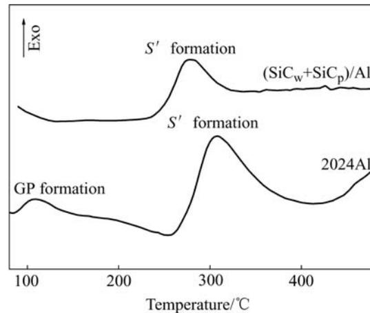
Fig.3 Comparison of DSC traces of solutionized 2024Al and hybrid composites
