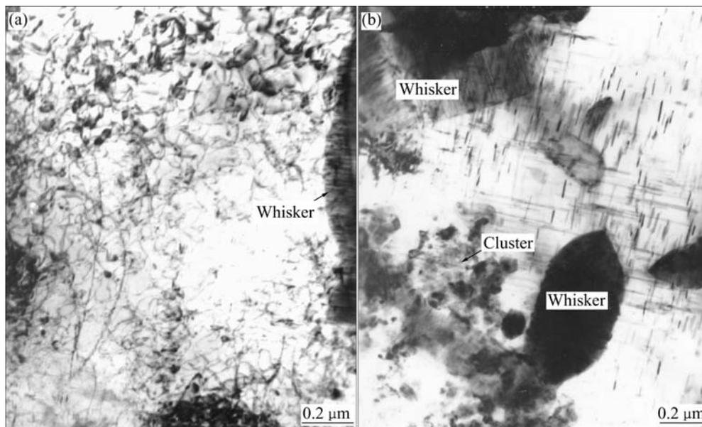
**Fig.4** TEM micrographs of  $(\text{SiC}_w+\text{SiC}_p)/2024\text{Al}$  composites aged at  $190\text{ }^\circ\text{C}$  for various times: (a) 2 h; (b) 5 h
