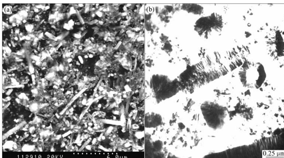
Fig.1 Microstructures of hybrid composites showing distribution of whiskers and nanoparticles by SEM(a) and TEM(b)
