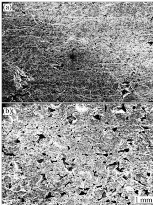
**Fig.3** SEM images of vertical section of foams compressed: (a) Quasi-static loading; (b) Dynamic loading
