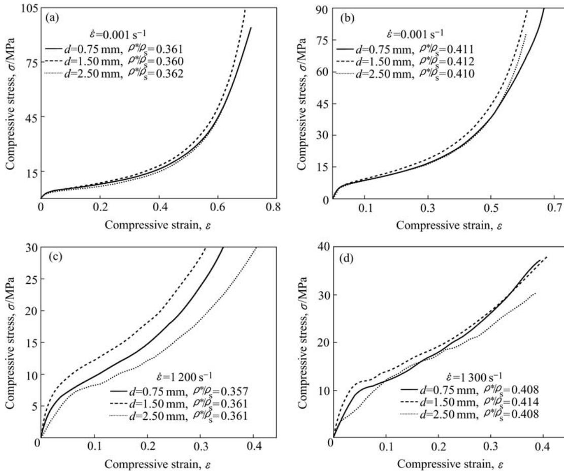
**Fig.2** Compressive stress-strain curves of aluminum foams of different cell sizes under quasi-static((a) and (b)) and dynamic loading (c) and (d)) conditions with  $\rho^*/\rho_s \approx 0.36$  and  $0.41$  respectively
