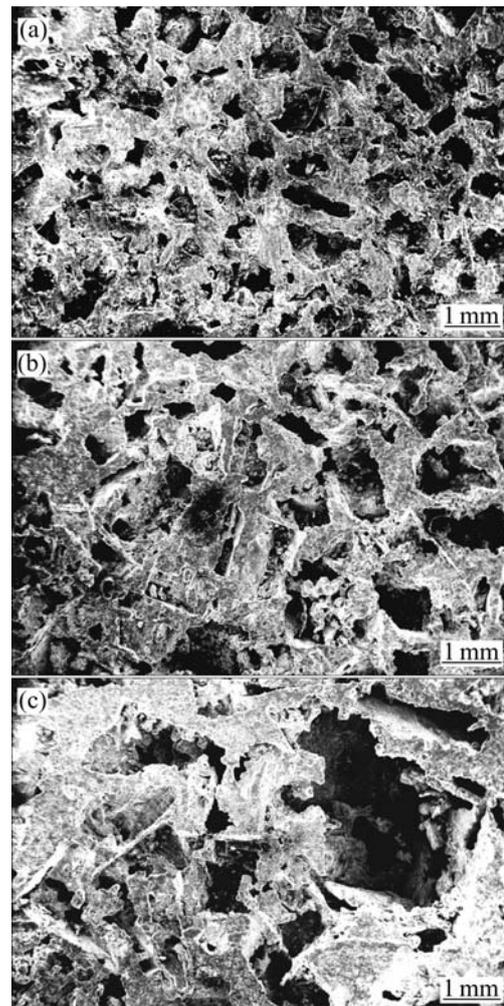
**Fig.1** Microstructures of aluminum foams with different cell sizes: (a) 0.75 mm; (b) 1.50 mm; (c) 2.50 mm
