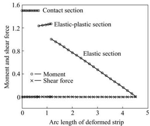
**Fig.7** Moment and shear force of deformed thin strip of model 1
