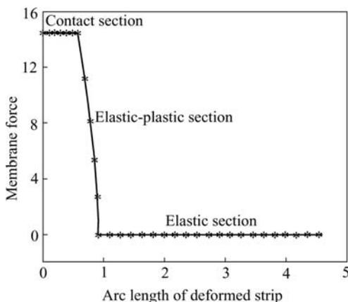
Fig.10 Membrane force of deformed thin strip of model 2
