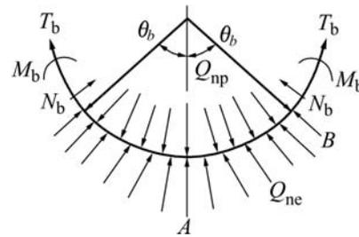
Fig.3 Mechanical model for contact part *AB*
