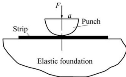
Fig.1 Stamping thin strip on elastic foundation
