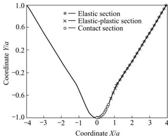
**Fig.5** Deflection process and shape of thin strip of model 1
