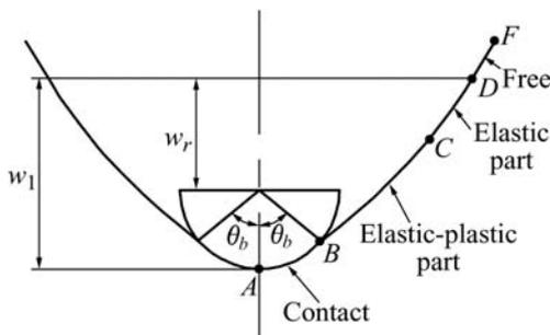
Fig.2 Deformation process and four parts of thin strip
