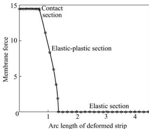
Fig.9 Membrane force of deformed thin strip of model 1
