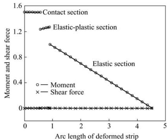
**Fig.8** Moment and shear force of deformed thin strip of model 2
