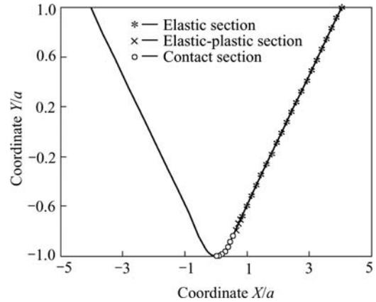
**Fig.6** Deflection process and shape of thin strip of model 2
