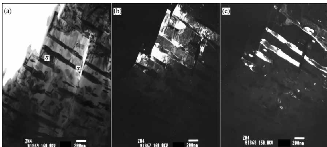
Fig.6 Images of lamellar structure of \beta phase decomposition in like-eutecticum of ZA-27 alloy aged for 5 h: (a) Bright field image; (b) Dark field image of \eta ; (c) Dark field image of \alpha
