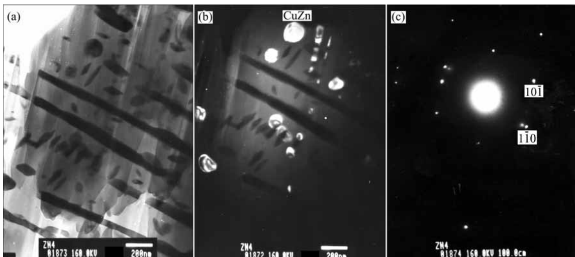
Fig. 9 TEM images of lamellar structure and electron diffraction pattern of CuZn in like-eutecticum of SiCp/ZA-27 composite aged for 5 h: (a) Bright field image; (b) Dark field image; (c) Electron diffraction pattern of CuZn in [111]
