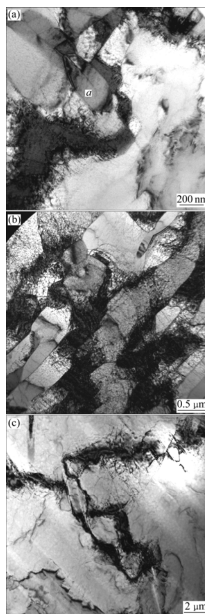
Fig.2 TEM images of cold-swaged TNTZO alloy annealed at 800 °C for 5 min
