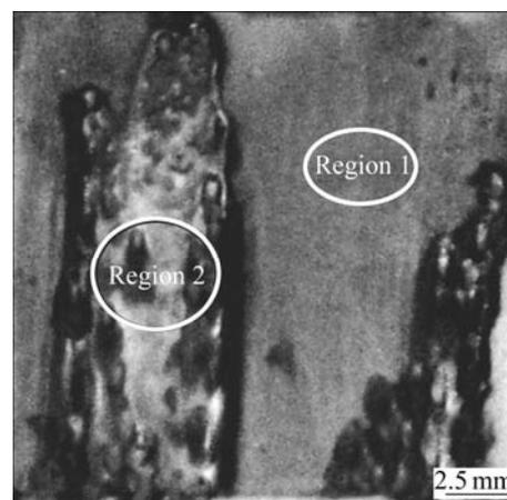
**Fig.3** Optical image of surface morphology after salt spray corrosion for 240 h
