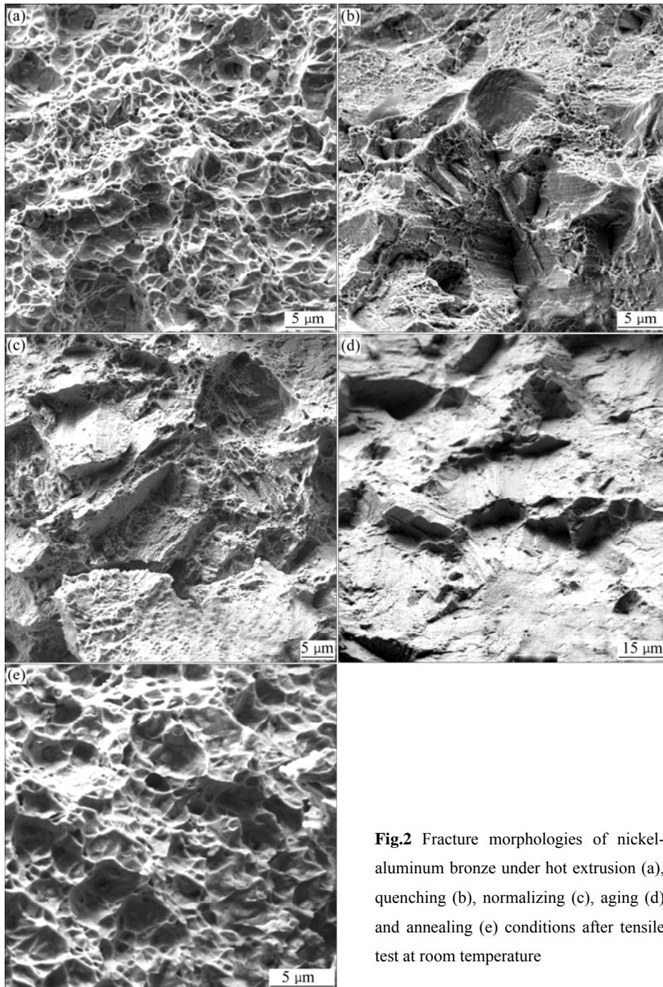
**Fig.2** Fracture morphologies of nickel-aluminum bronze under hot extrusion (a), quenching (b), normalizing (c), aging (d) and annealing (e) conditions after tensile test at room temperature
