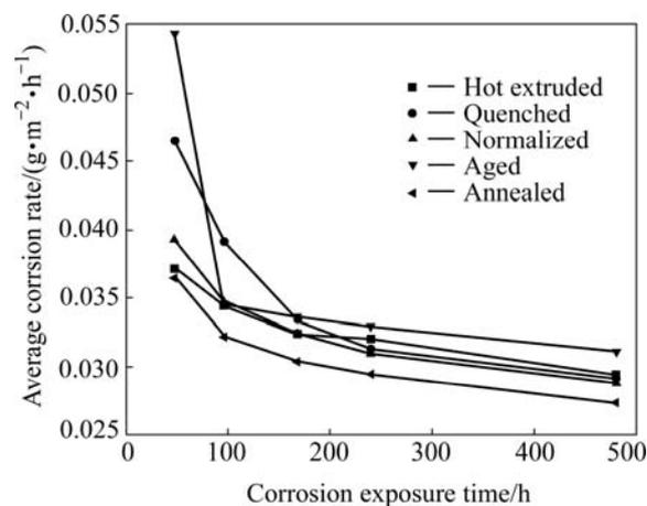
**Fig.4** Change of average corrosion rate of nickel-aluminum bronze exposed to salt spray environment with exposure time
