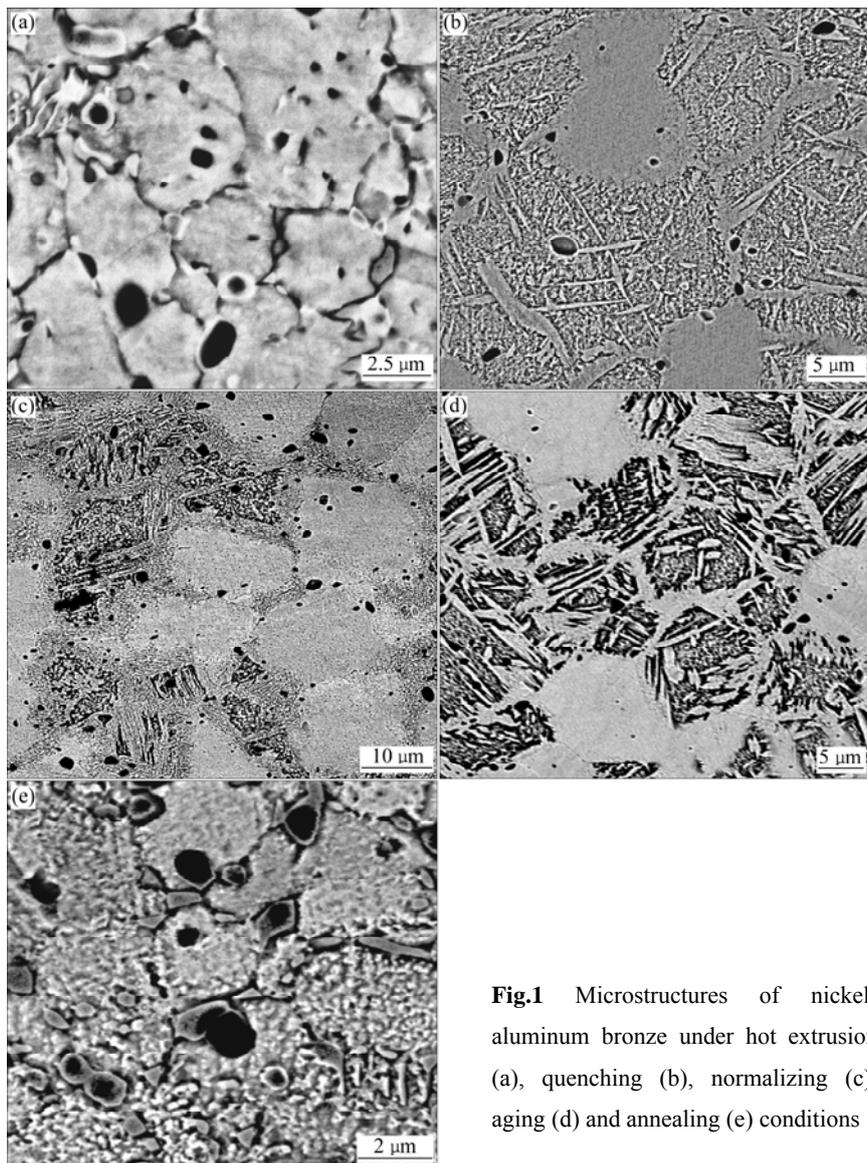
**Fig.1** Microstructures of nickel-aluminum bronze under hot extrusion (a), quenching (b), normalizing (c), aging (d) and annealing (e) conditions
