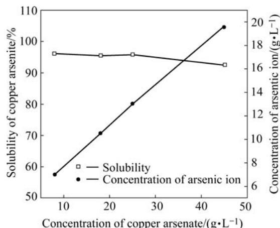
**Fig.7** Impacts of copper arsenite concentration on its solubility and concentration of arsenic ion
