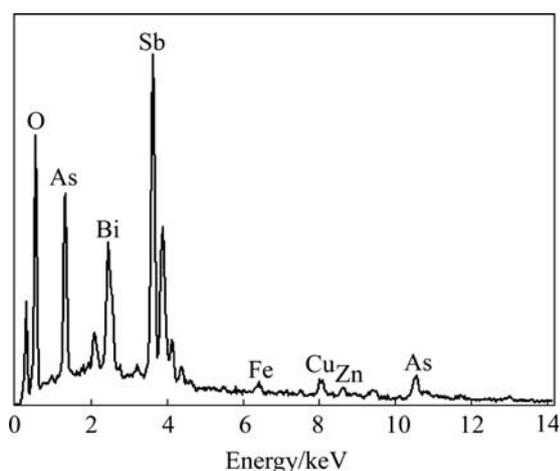
Fig.10 EDX pattern of yellow precipitate
