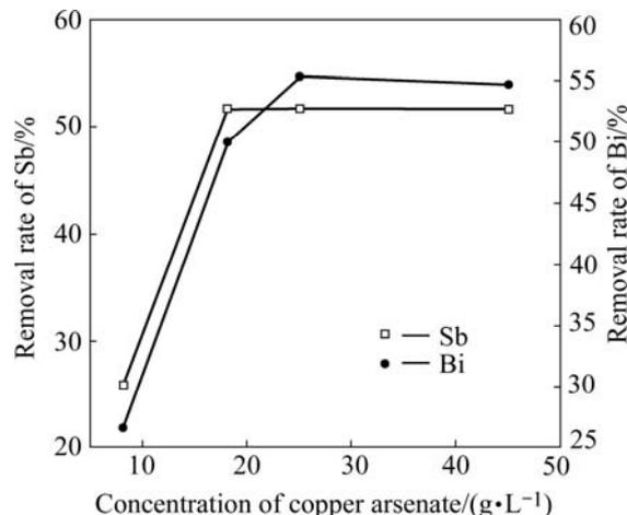
**Fig.8** Impacts of copper arsenite concentration on removal rate of Sb and Bi
