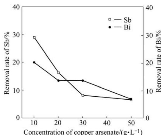
**Fig.4** Impacts of copper arsenate concentration on removal rate of Sb and Bi
