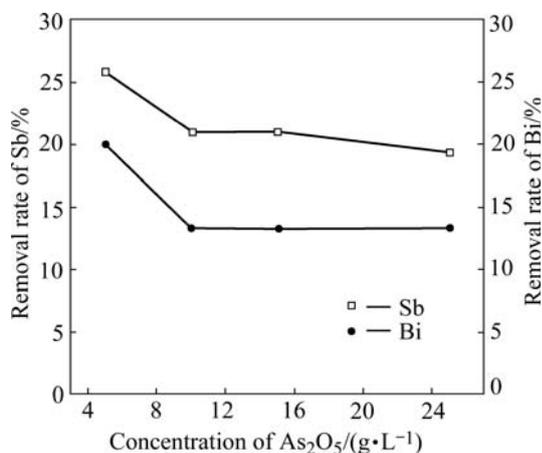
**Fig.2** Impacts of  $As_2O_5$  concentration on removal rate of Sb and Bi
