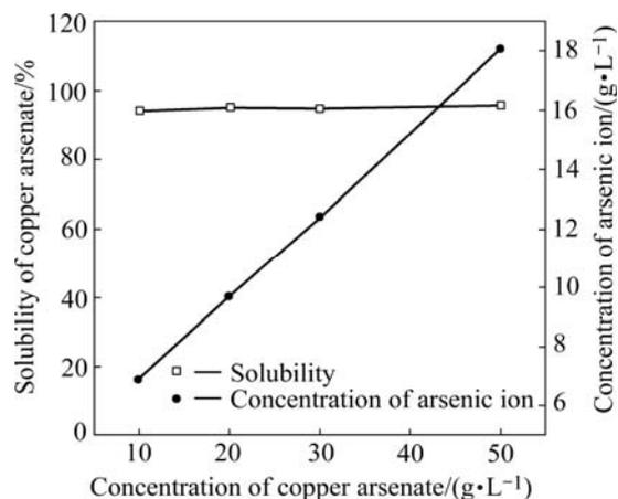
**Fig.3** Impacts of copper arsenate concentration on its solubility and concentration of arsenic ion
