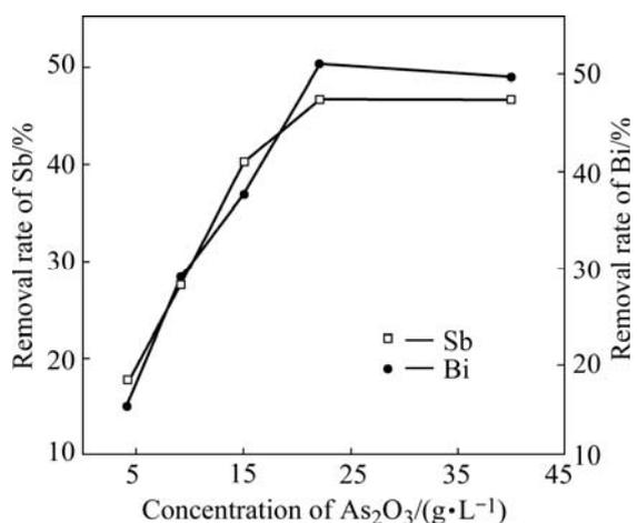
**Fig.6** Impacts of  $As_2O_3$  concentration on removal rate of Sb and Bi
