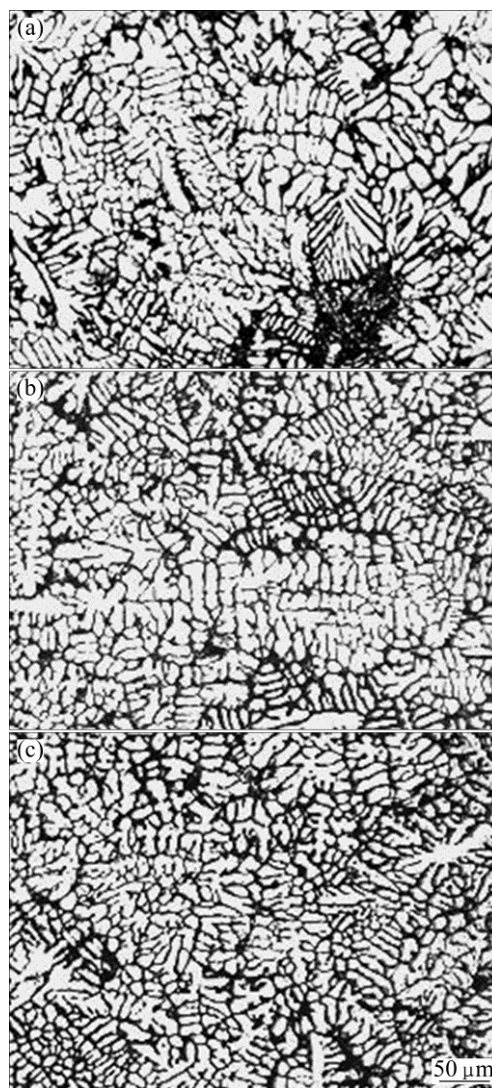
Fig. 4 Microstructures of as-cast alloys: (a) Alloy A319 (0.3% Mg); (b) Alloy TH1(1.0% Mg); (c) Alloy TH2 (1.5%Mg)
