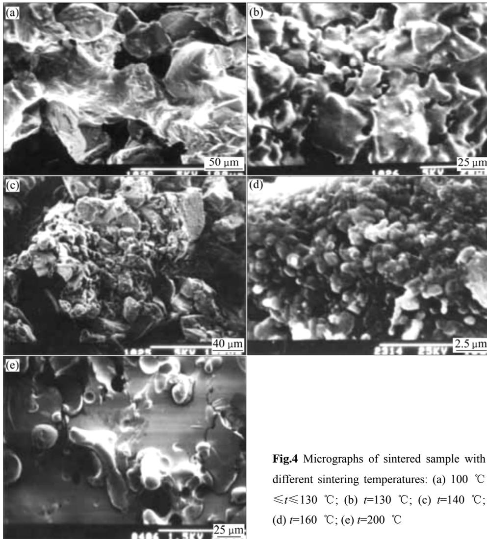
**Fig.4** Micrographs of sintered sample with different sintering temperatures: (a) 100 °C  $\leq t \leq 130$  °C; (b)  $t=130$  °C; (c)  $t=140$  °C; (d)  $t=160$  °C; (e)  $t=200$  °C
