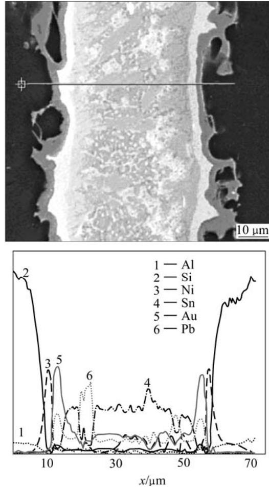
**Fig.8** SEM photograph and element distributions of solderable coating of Si-Al alloy
