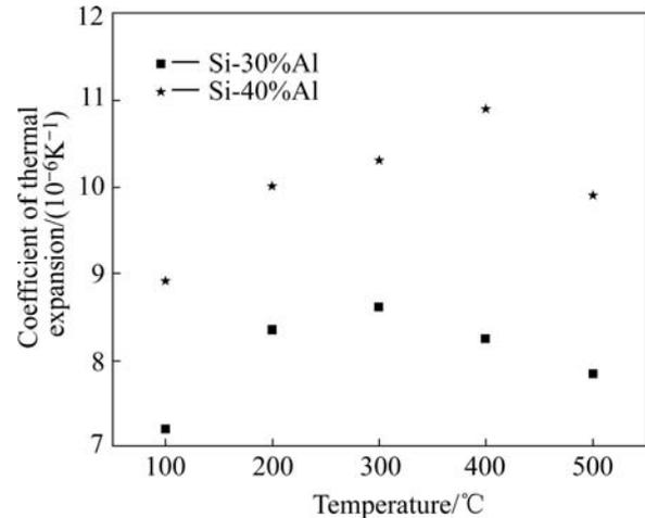
**Fig.2** Coefficient of thermal expansion of spray formed Si-Al alloys after hot pressing
