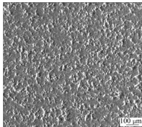
**Fig.6** SEM photograph of densified Si-Al alloy after gold plating
