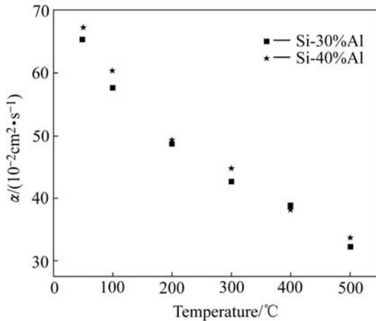
**Fig.4** Thermal diffusivity of spray formed Si-Al alloys after hot pressing
