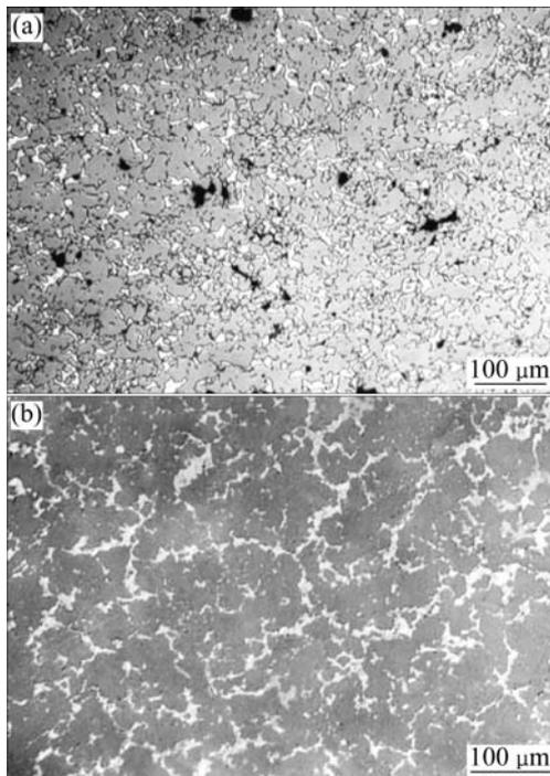
**Fig.1** Microstructures of spray formed Si-30%Al alloy: (a) As-deposited; (b) After hot pressing
