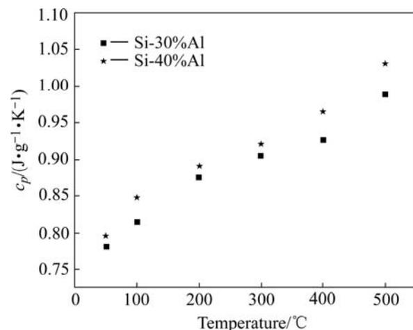
**Fig.3** Heat capacity of spray formed Si-Al alloys after hot pressing
