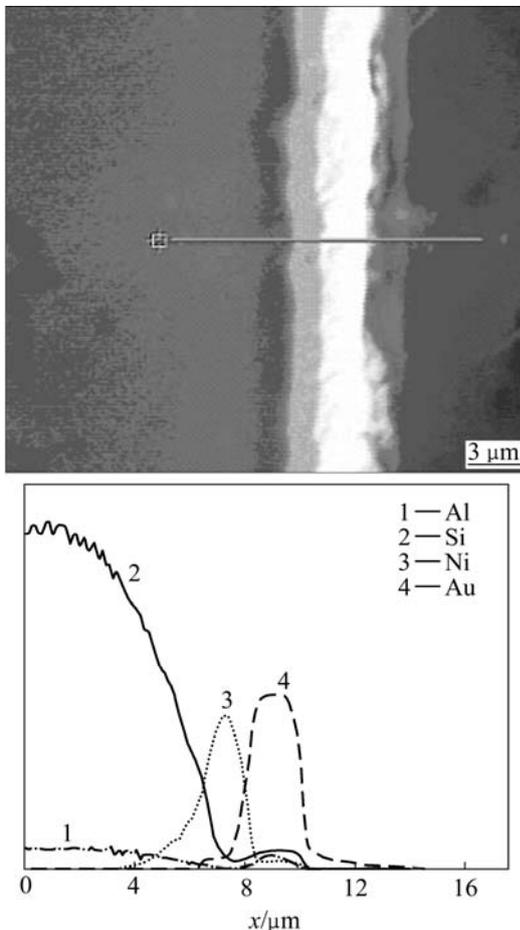
**Fig.7** SEM photograph and element distributions of plating of Si-Al alloy
