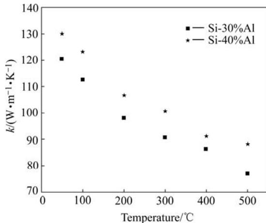
**Fig.5** Thermal conductivity of spray formed Si-Al alloys after hot pressing
