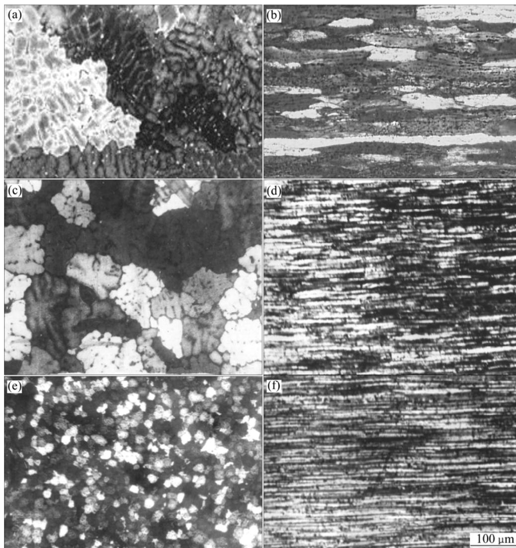
**Fig.1** Optical microstructures of studied alloys: (a) Alloy A, as-cast; (b) Alloy A, as-solution; (c) Alloy B, as-cast; (d) Alloy B, as-solution; (e) Alloy C, as-cast; (f) Alloy C, as-solution
