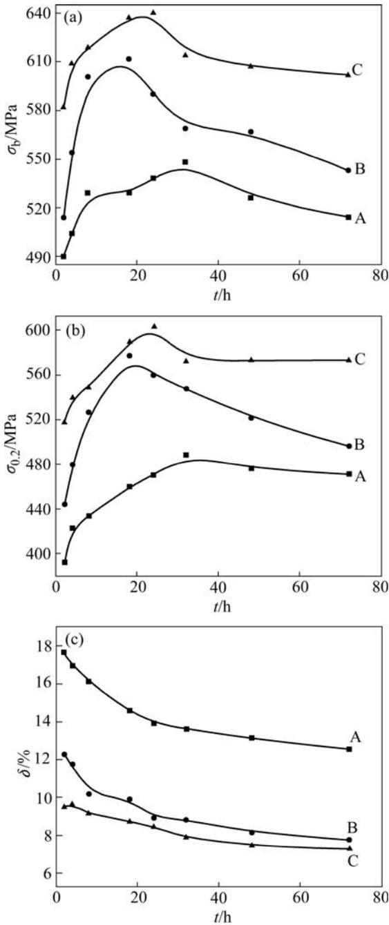
**Fig.3** Mechanical properties of studied alloys aged at 120 °C for various times: (a)  $\sigma_b-t$ ; (b)  $\sigma_{0.2}-t$ ; (c)  $\delta-t$
