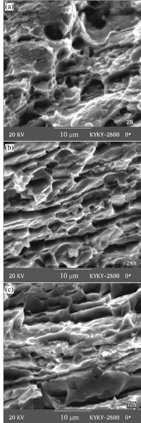
**Fig.4** SEM images of fracture surfaces of alloy C aged for various times: (a) Aging 120 °C, 2 h; (b) Aging 120 °C, 24 h; (c) Aging 120 °C, 72 h
