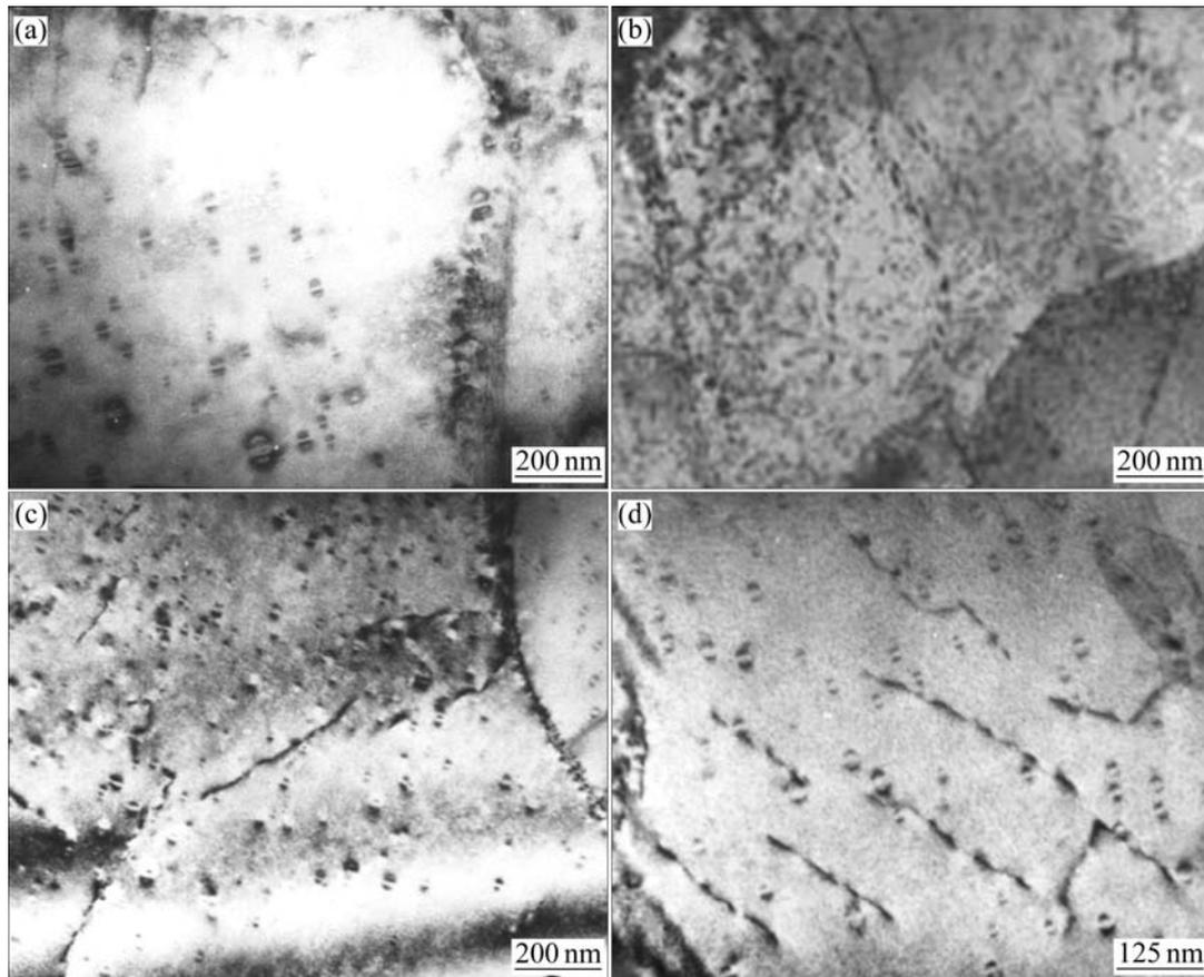
**Fig.2** TEM images of alloy C at 120 °C ageing for 24 h: (a), (b) Dispersed particles; (c), (d) Pinned dislocations
