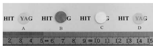
Fig.4 Appearance of samples sintered in vacuum (specification described in Table 1)
