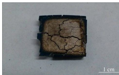
Fig. 2 Cracks on surface of hydrogenated pure titanium cast ingot sample
