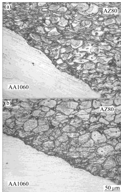
**Fig. 6** Micrographs of transversely sectioned composite bars produced at 250 °C (a) and 300 °C (b) in vicinity of interface of two alloys
