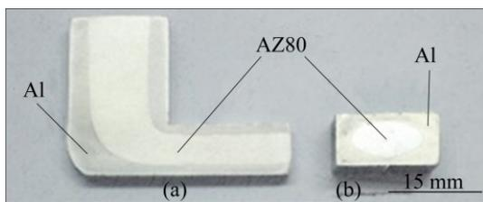
**Fig. 5** Longitudinal (a) and transverse (b) sections of NECLE-treated composite specimen
