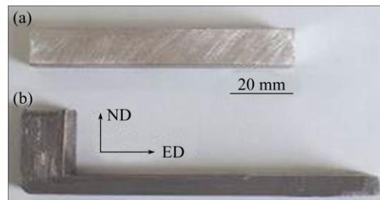
Fig. 3 Billet (a) together with specimen partially deformed by NECLE process (b)
