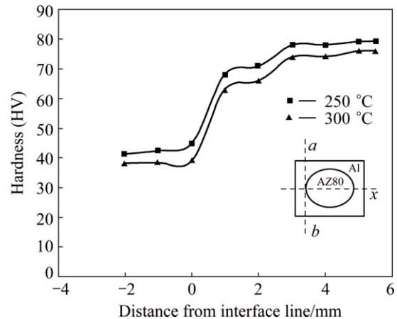
**Fig. 9** Distributions of hardness in  $x$  direction and in terms of distance from  $ab$  interface line of bimetal bars produced at various temperatures
