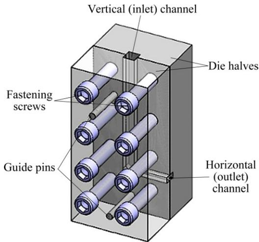
Fig. 1 Schematic illustration of assembled NECLE die
