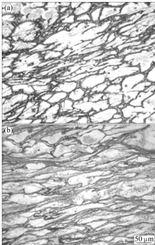
**Fig. 7** Longitudinal views of microstructures of AZ80 cores of bimetal components deformed at 250 °C (a) and 300 °C (b)
