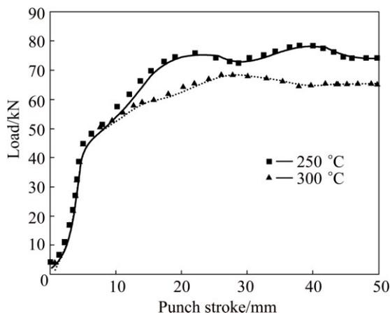
**Fig. 10** Load–stroke curves of bimetal NECLE operations conducted at 250 and 300 °C
