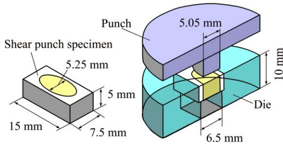
**Fig. 4** Schematic diagrams of composite sample and die set up for evaluation of interfacial shear strength
