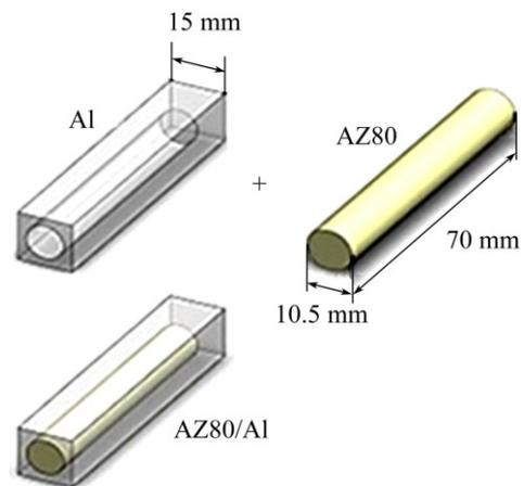
Fig. 2 General dimensions of Al sheath and AZ80 core together with composite billet
