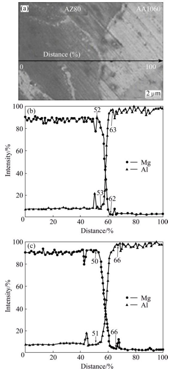
**Fig. 8** Results of line scan analyses at AZ80/Al interface (a) of composite products NECLE-treated at 250 °C (b) and 300 °C (c)
