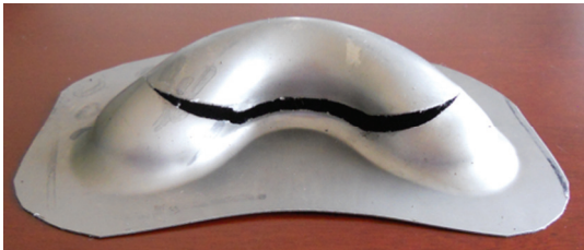
图 3 坯料不合理导致的破裂试件 Fig. 3 Rupture specimen based on unreasonable blank
