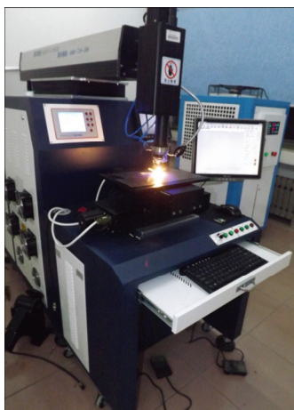
Fig. 4 Apparatus of TWB laser welding processing
