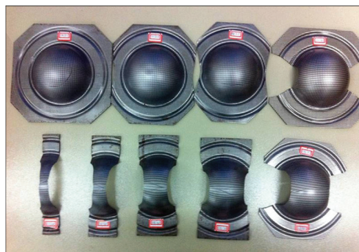
Fig. 10 Formed samples after failure in hemispherical punch bulging tests
