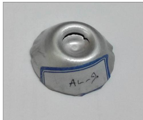
**Fig. 14** Aluminum blank with initial diameter of 50 mm and thickness of 1.1 mm after forming process using PVC Teflon-filler
