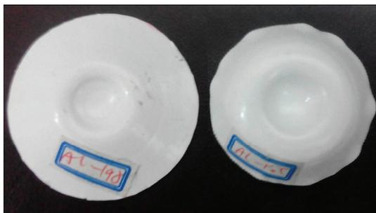
**Fig. 16** Two aluminum blanks P01-AL150-W and P07-AL150-W with diameter of 50 mm and thickness of 1.5 mm after forming process
