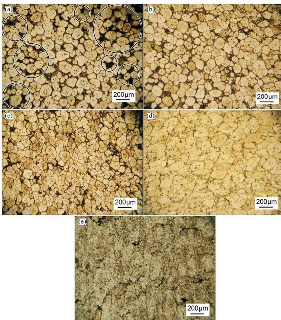
Fig. 6 Microstructures of thixoformed component in different positions (specific pressure of 250 MPa and base thickness of 3 mm): (a) Position 1; (b) Position 2; (c) Position 3; (d) Position 4; (e) Position 5
