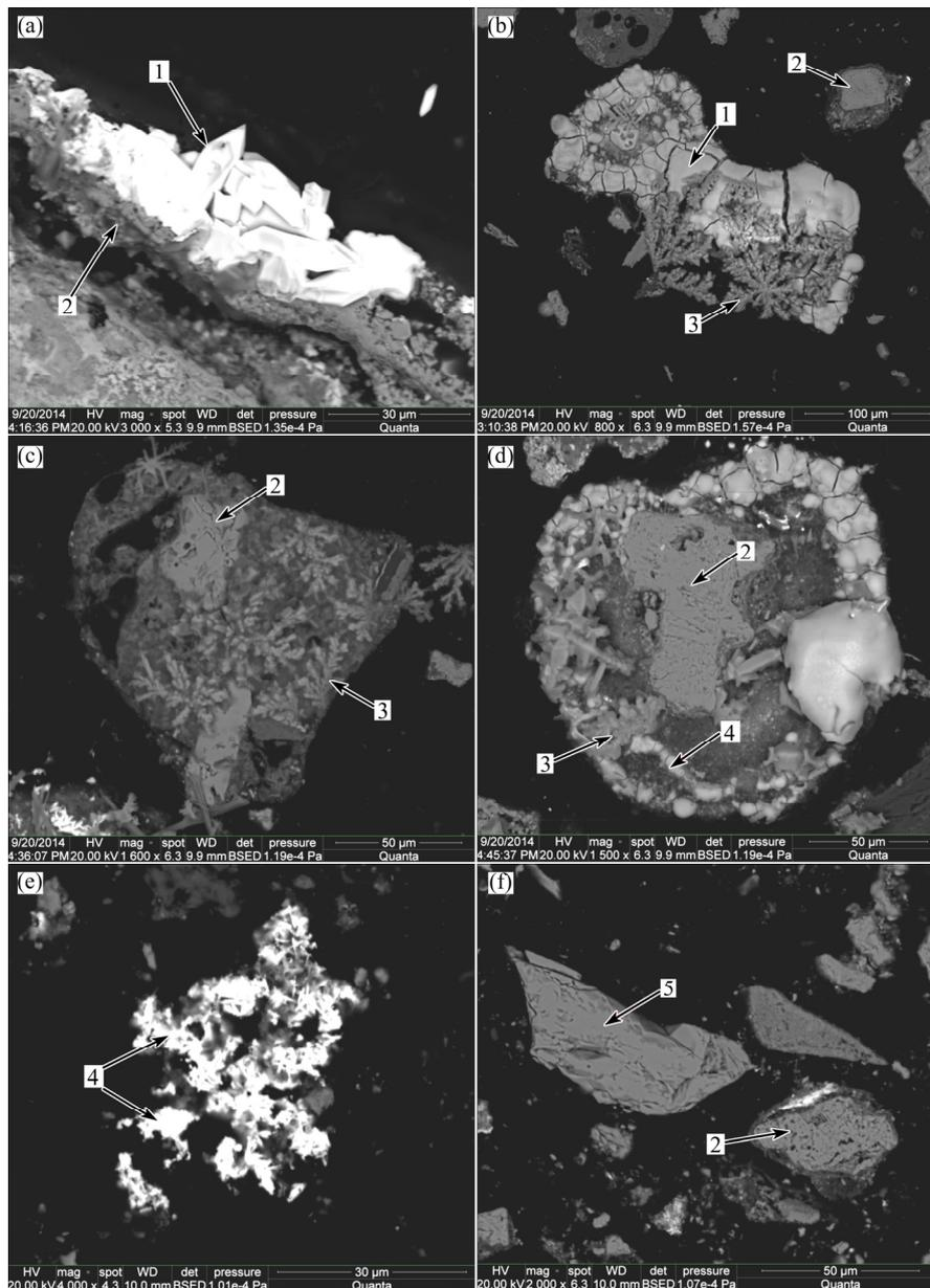
**Fig. 3** SEM images of sintering dust before and after grinding: (a) Pseudocotunnite particle on hematite particle; (b) Lead bearing particle with KCl coat; (c) Hematite particle with KCl coat; (d) Hematite particle enwrapped by lead bearing particle with KCl coat; (e) Lead-bearing particles after wetting grinding; (f) Iron-bearing particles after wetting grinding (1—Pseudocotunnite; 2—Hematite; 3—KCl; 4—Lead-bearing particle; 5—Magnetite)
