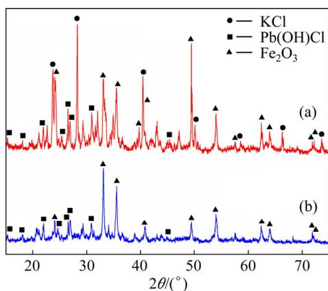
Fig. 2 X-ray diffraction patterns of sintering dust before (a) and after (b) wetting grinding
