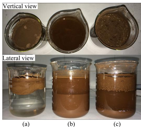
**Fig. 4** Dispersibility and wettability of sintering dust under different treatments: (a) No pretreatment; (b) Wetting grinding for 2 min; (c) Agitating at 400 r/min for 10 min (every treatment has a solid-to-liquid ratio of 1:2.5 and stands for 15 min)
