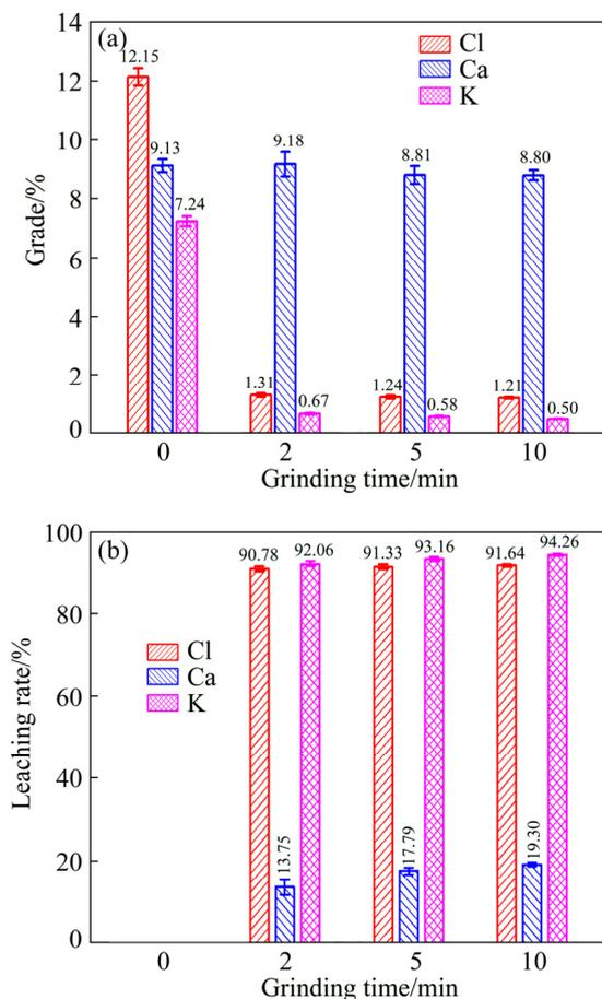
Fig. 7 Effects of wetting grinding on residual grade (a) and leaching rate (b) of Cl, Ca and K in sintering dust
