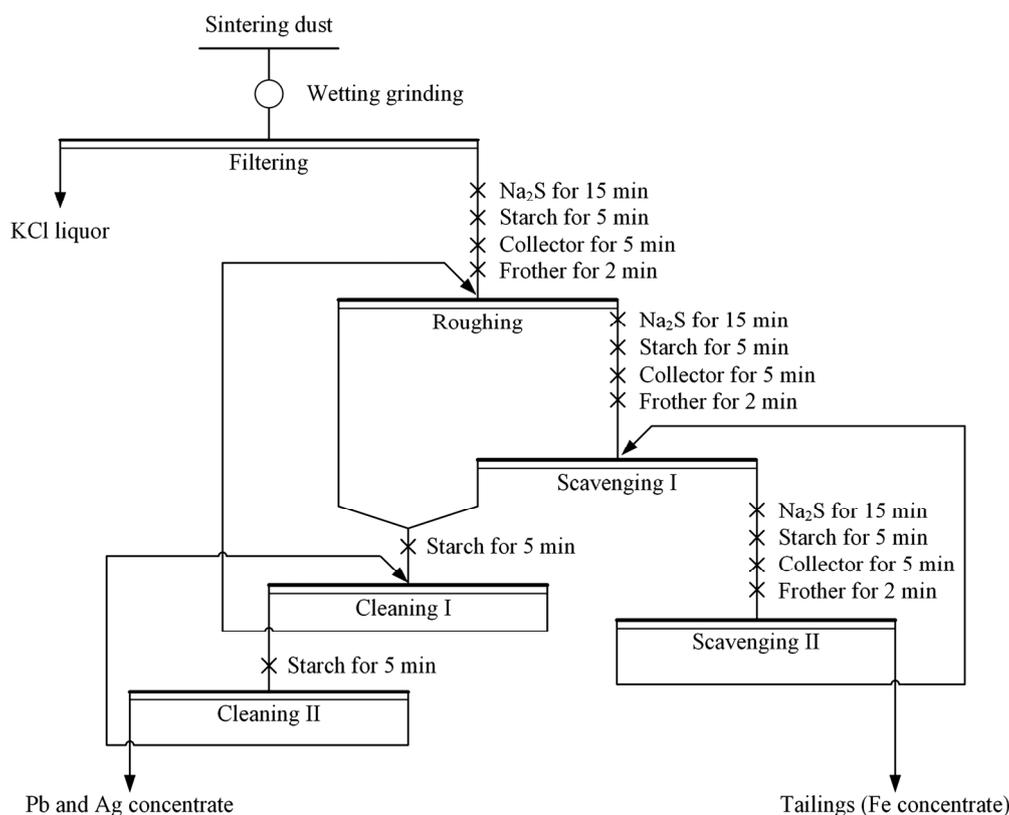
Fig. 1 Wetting grinding and flotation flowsheet for closed-circuit process of sintering dust
