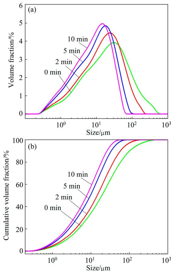
Fig. 6 Effects of wetting grinding on size of sintering dust
