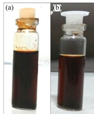
Fig. 5 Photos of dispersion of synthesized copper nanoparticles before (a) and after (b) two months of storage
