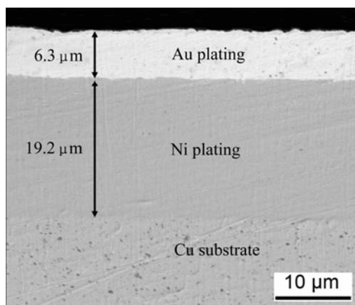
Fig. 1 SEM image of Au plating
