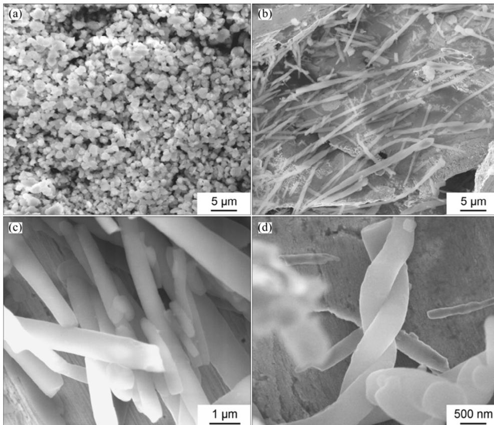
**Fig. 7** SEM images of typical wear debris: (a) Particle wear debris; (b) Roller-shaped wear debris; (c,d) High magnification images of roller-shaped and twist-shaped wear debris in (b), respectively
