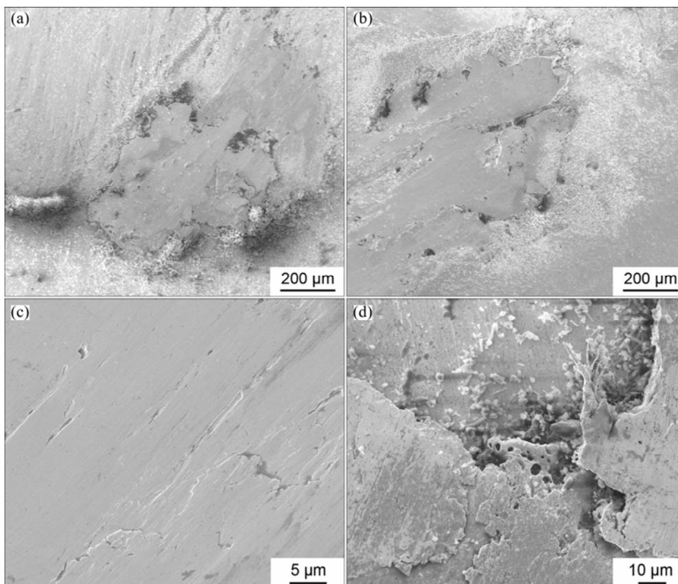
**Fig. 5** SEM images of worn surfaces of AuAgCu brushes at loads of 0.4 N (a) and 0.8 N (b), typical center (c) and edge (d) regions of worn surface of (b)
