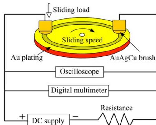
Fig. 2 Schematic diagram of brush-on-disc contact and electrical circuit
