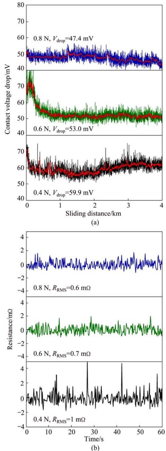
**Fig. 3** Effects of normal load on contact voltage drop (a) and resistance waveform (b)
