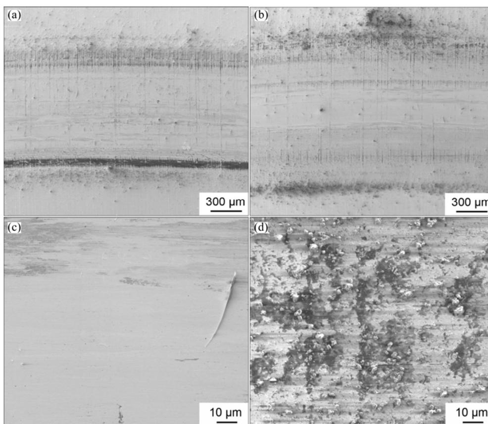
**Fig. 6** SEM images of wear tracks of Au plating at loads of 0.4 N (a) and 0.8 N (b), typical center (c) and edge (d) regions of wear track of (b)
