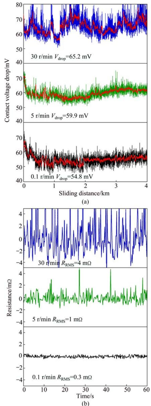
**Fig. 4** Effects of sliding speed on contact voltage drop (a) and resistance waveform (b)
