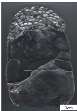
Fig. 3 Vertical section of aluminum foam produced by air and nitrogen sequentially
