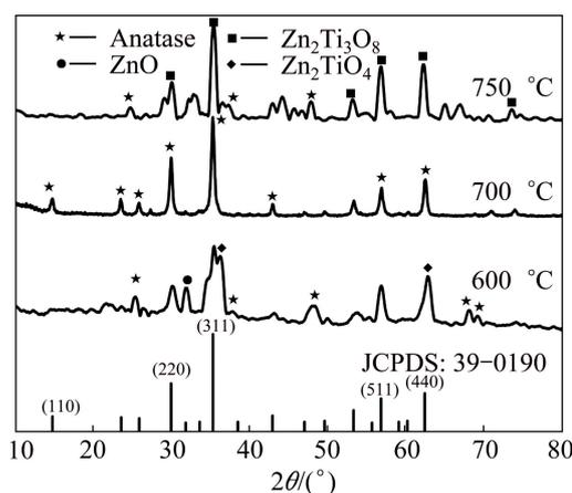
**Fig. 4** XRD patterns of samples calcined in air at different temperatures
