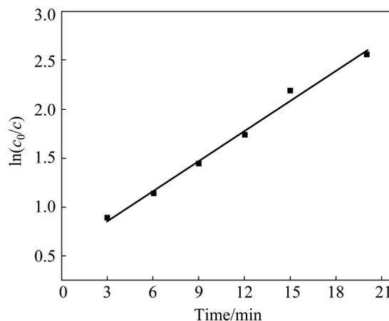
**Fig. 9** Kinetics curve of photocatalyst degradation
