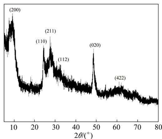
Fig. 1 XRD pattern of protonated titanates
