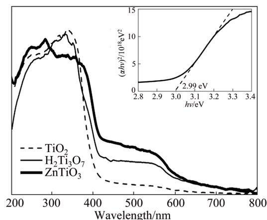
**Fig. 6** DRS for  $\text{TiO}_2$ ,  $\text{H}_2\text{Ti}_3\text{O}_7$  and  $\text{ZnTiO}_3$  (inset shows estimated band gap of chain-like  $\text{ZnTiO}_3$ )
