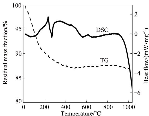
**Fig. 3** Results of thermal analysis of zinc titanate precursor
