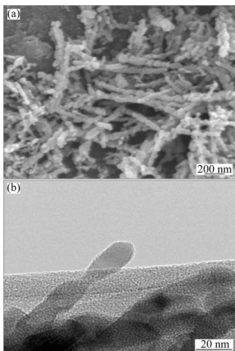
**Fig. 5** SEM (a) and TEM (b) images of chain-like  $\text{ZnTiO}_3$  specimens
