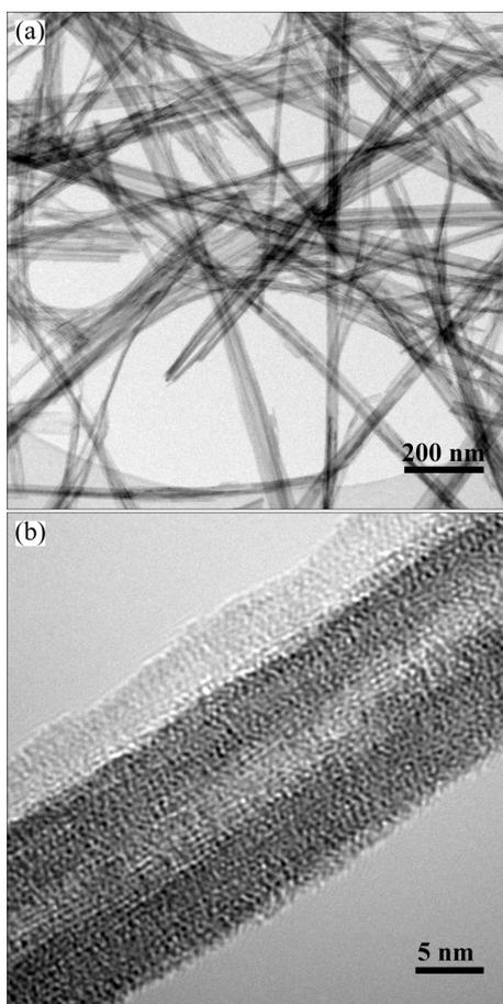
**Fig. 2** TEM images of  $\text{H}_2\text{Ti}_3\text{O}_7 \cdot 3\text{H}_2\text{O}$  nanotube structures: (a) Low magnification; (b) High magnification
