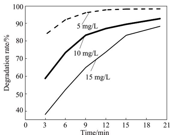
**Fig. 8** Effect of initial methyl orange concentration on degradation rate of methyl orange
