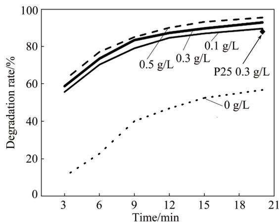
**Fig. 7** Effect of ZnTiO<sub>3</sub> concentration on degradation rate of methyl orange and comparison with commercial catalyst P25
