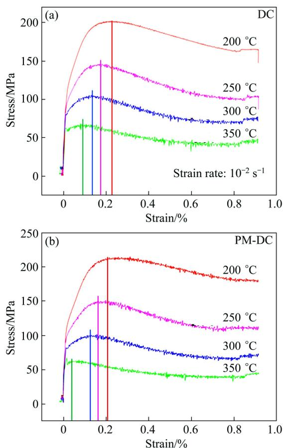
**Fig. 7** True stress–strain curves of DC (a) and PM-DC (b) casting ingots of AZ80 alloy at different temperatures
