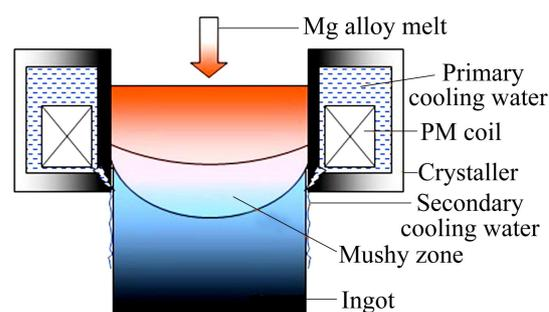
**Fig. 1** Schematic diagram of DC casting under condition of LVPMF (PM-DC)
