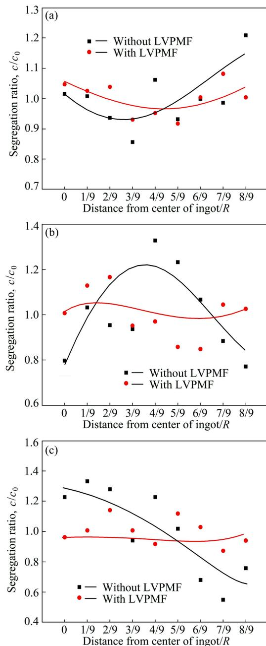
**Fig. 4** Macro segregation of main solute elements Al, Zn and Mn in AZ80 alloy ingots : (a) Al ; (b) Zn ; (c) Mn
