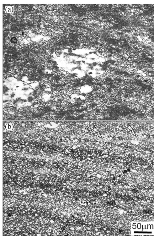
**Fig. 6** Deformation microstructures after upsetting of ingots: (a) DC; (b) PM-DC
