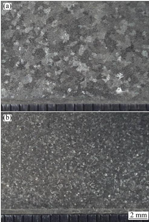
**Fig. 2** Macrostructures of DC casting ingots of AZ80 alloy with or without application of LVPMF: (a) DC; (b) PM-DC
