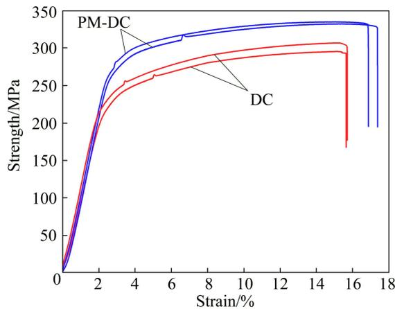
Fig. 8 Tensile properties of as-extruded AZ80 alloy
