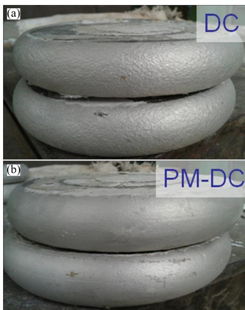
**Fig. 5** Slabs prepared by forging hammer process: (a) DC; (b) PM-DC
