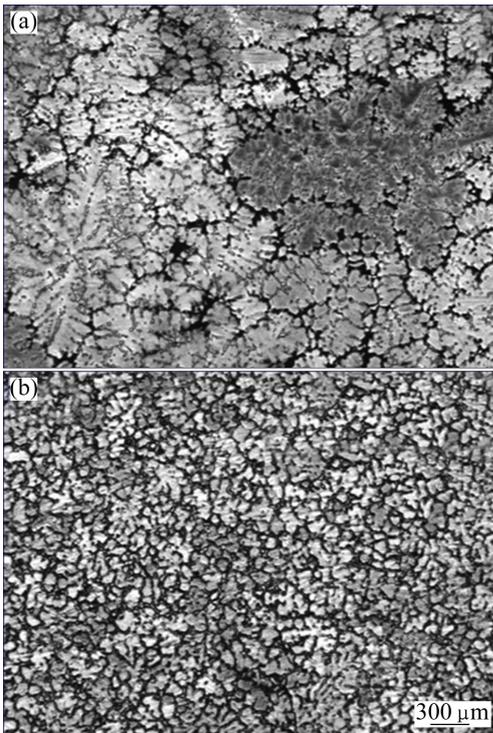
**Fig. 3** Microstructures of DC casting ingots of AZ80 alloy with or without application of LVPMF: (a) DC; (b) PM-DC
