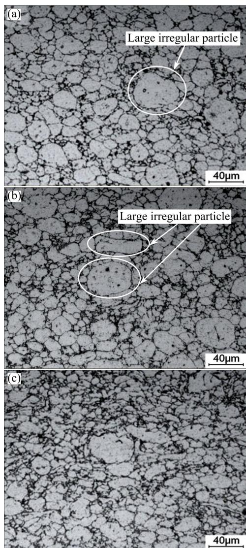
**Fig. 8** OM micrographs of 6061 alloys heated for 20 min at 650 °C (a), 655 °C (b) and 665 °C (c)
