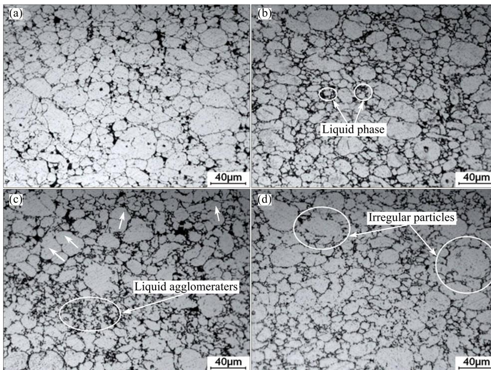
**Fig. 6** OM micrographs of the first region (small-sized powders) of 6061 alloys heated at 660 °C for 10 min (a), 20 min (b), 30 min (c) and 60 min (d)
