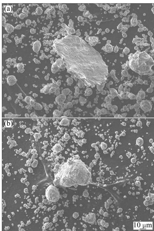
**Fig. 2** SEM micrographs of ball-milled powders (a) and un-milled powders (b) of 6061 alloy
