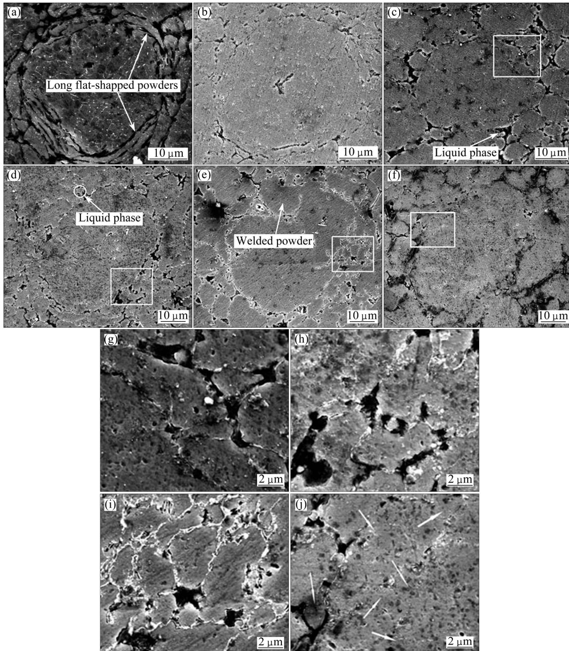
**Fig. 4** SEM micrographs of 6061 alloys heated at 660 °C for 0 min (a), 2 min (b), 5 min (c), 20 min (d), 30 min (e) and 60 min (f), respectively; (g–j) Enlarged micrographs corresponding to rectangular regions in Figs. (c)–(f) respectively
