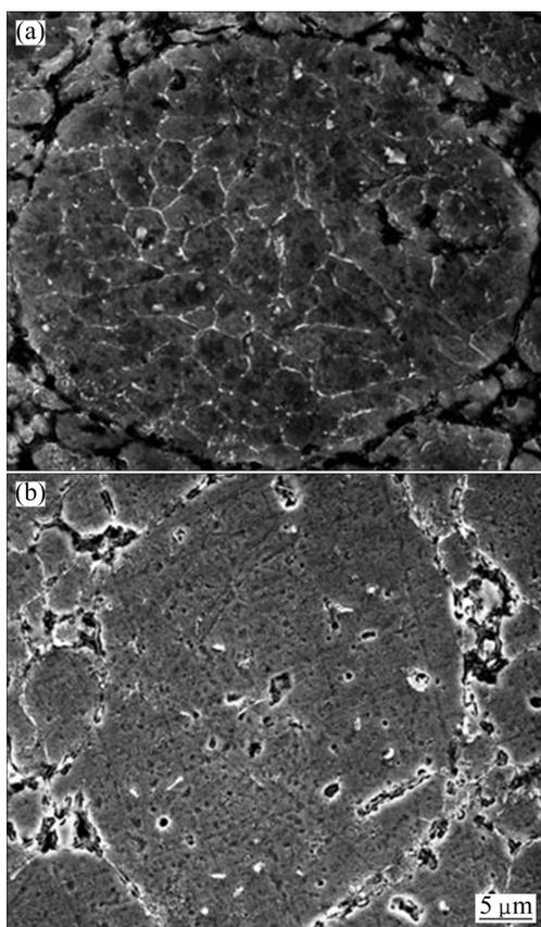
**Fig. 5** SEM micrographs of 6061 alloys composed of un-milled powders heated at 660 °C for 0 (a) and 7 min (b)
