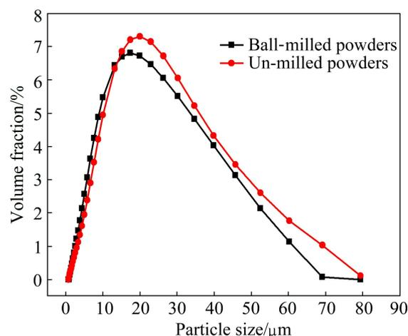
**Fig. 3** Particle size distributions of both ball-milled powders and un-milled powders
