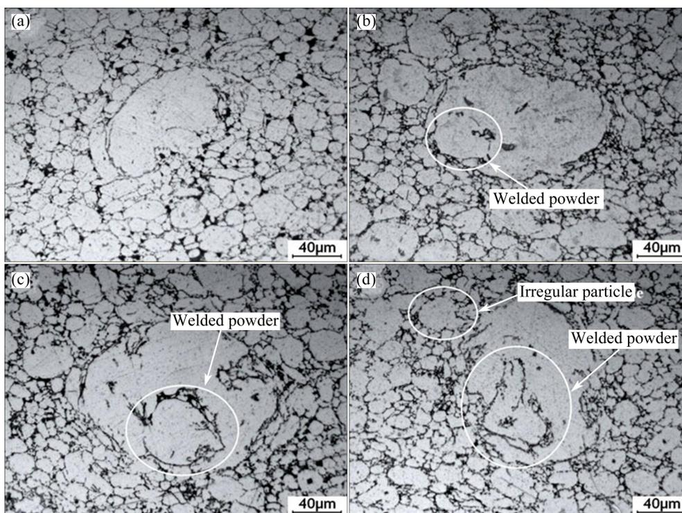
**Fig. 7** OM micrographs of the second region (large powders surrounded by long flat-shaped powders) of 6061 alloys heated at 660 °C for 10 min (a), 20 min (b), 30 min (c) and 60 min (d)
