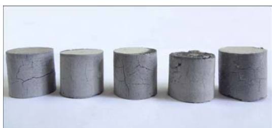
Fig. 4 Cracks of green bodies in process of low-temperature drying
