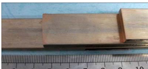
Fig. 4 TZCC Cu–4.7%Sn alloy plate (20 mm×5 mm) with smooth surface
