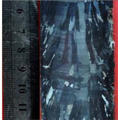
Fig. 1 Macrostructure of directionally solidified ingot
