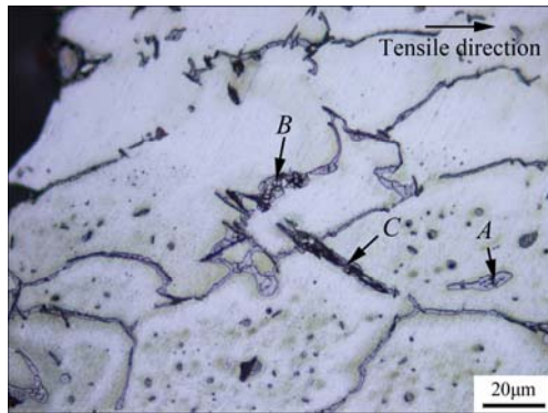
Fig. 11 Microstructure near fracture in crack initiation region
