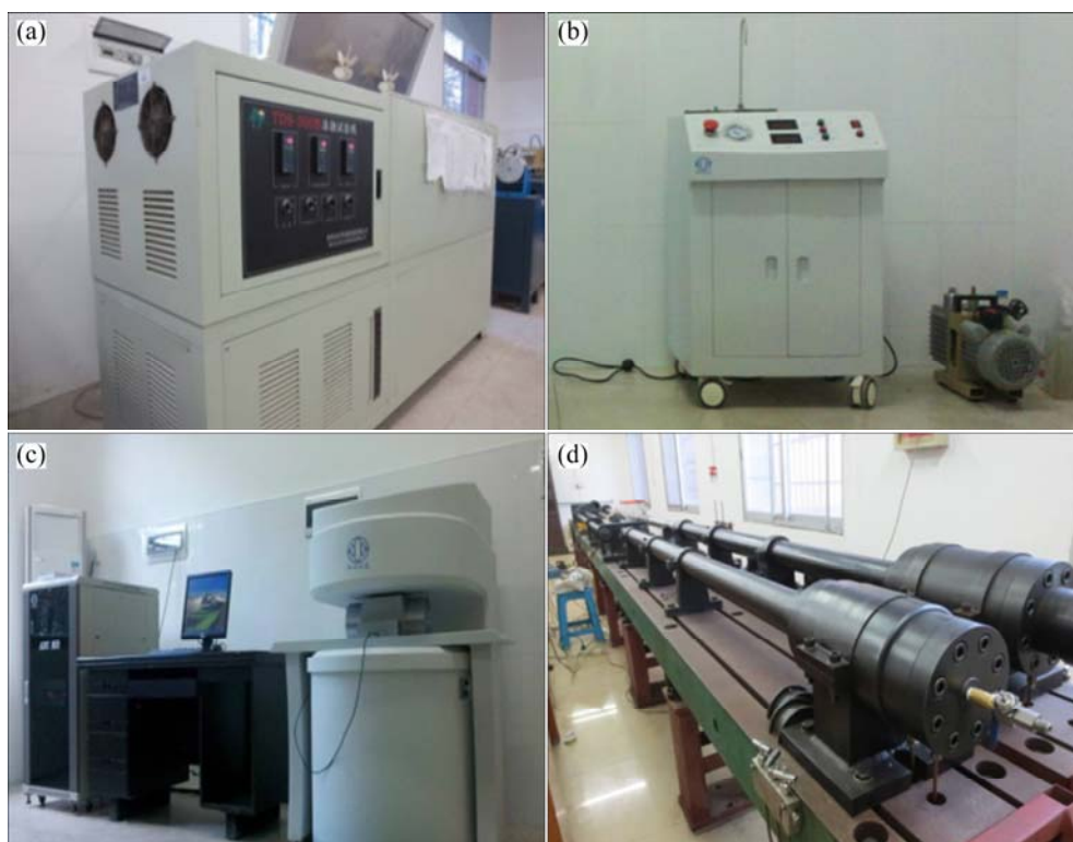
Fig. 2 Main experimental equipments: (a) freeze–thaw cycle test machine; (b) Vacuum saturation device; (c) NMR test system; (d) SHPB equipment
