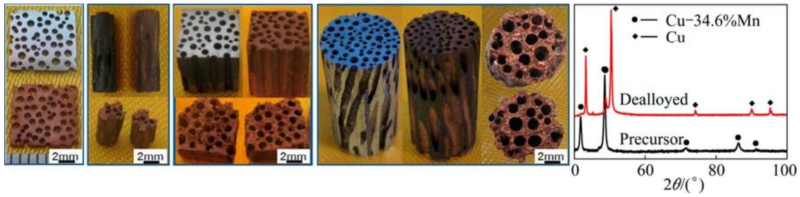
**Fig. 2** Gasar Cu–34.6%Mn alloy (silver white), hybrid porous structure (dark red) of different types, and XRD patterns before and after high temperature chemical dealloying [18]
