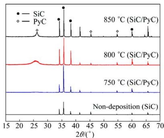
Fig. 1 XRD patterns of surface of SiC and SiC/PyC
