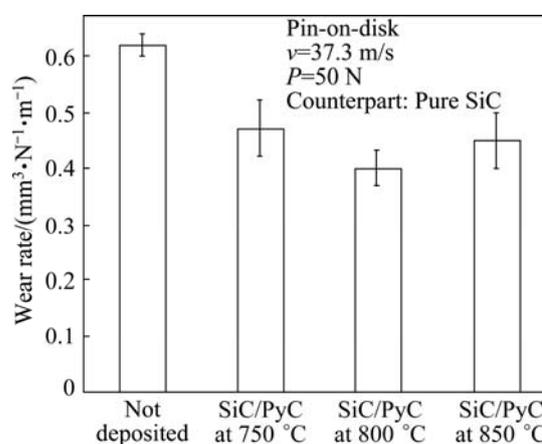
**Fig. 3** Effect of deposition temperature on wear rate of SiC and SiC/PyC under dry sliding condition
