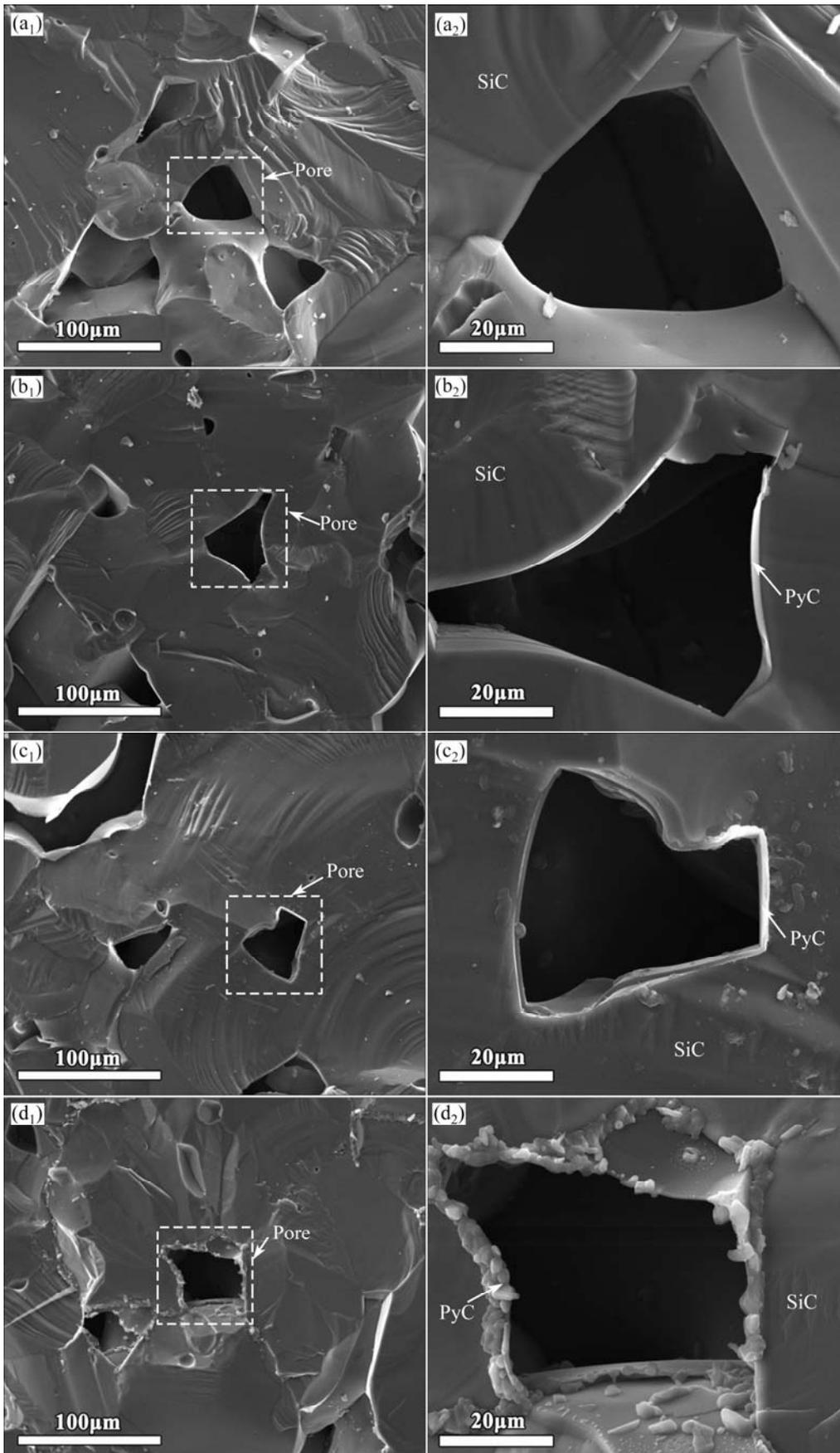
**Fig. 2** SEM images of cross section of SiC/PyC composite materials: (a<sub>1</sub>–d<sub>1</sub>) Morphologies of cross section of pure SiC and PyC/SiC produced by CVI at 750, 800 and 850 °C, respectively; (a<sub>2</sub>–d<sub>2</sub>) Local area magnification images of (a<sub>1</sub>–d<sub>1</sub>), respectively
