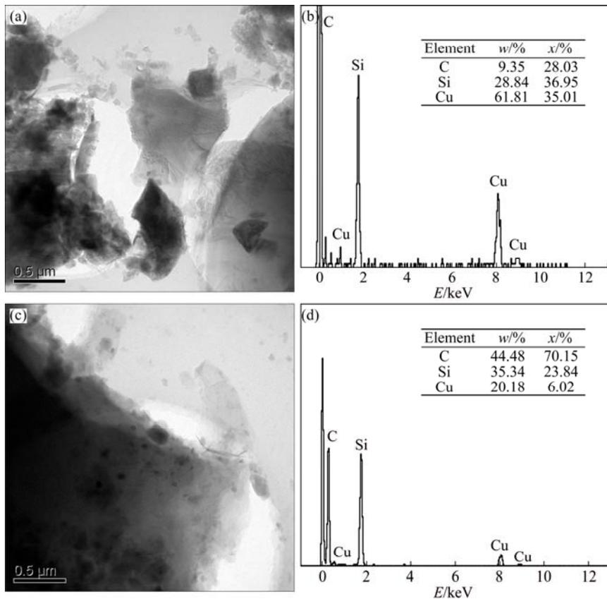
**Fig. 5** TEM images (a, c) and EDS analysis (b, d) of debris particles of SiC and SiC/PyC: (a, b) Pure SiC; (c, d) PyC/SiC produced by CVI at 800 °C
