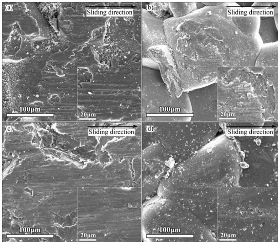
**Fig. 4** SEM images of worn surface: Morphologies of surface of pure SiC (a), PyC/SiC produced by CVI at 750 °C (b), 800 °C (c) and 850 °C (d)
