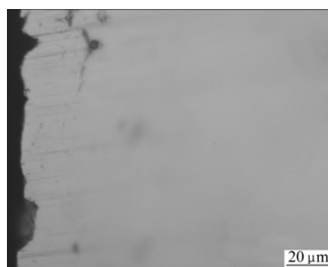
Fig. 2 Side view of brass immersed in sweat solution for 28 d
