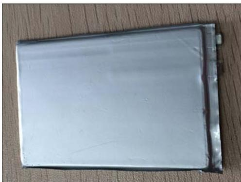
Fig. 4 Prototype of 053048 square Li ion battery
