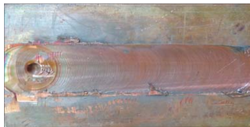
Fig. 4 Typical crown appearance of friction stir processed copper surface composites reinforced with B_4C particles
