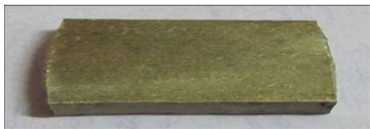
Fig. 10 Macrophotograph of designed alloy after hot rolling at 800 °C and 10 s -1
