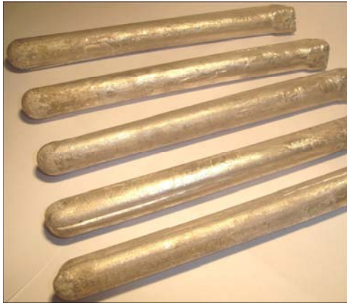
Fig. 2 Test samples of AS series magnesium alloys
