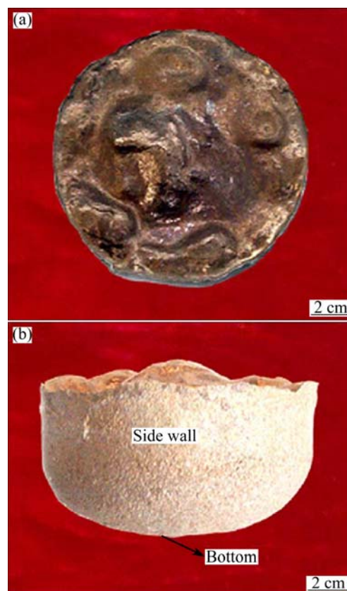
Fig. 1 Photographs of sample solidified inside CaO crucible: (a) Top view; (b) Side view
