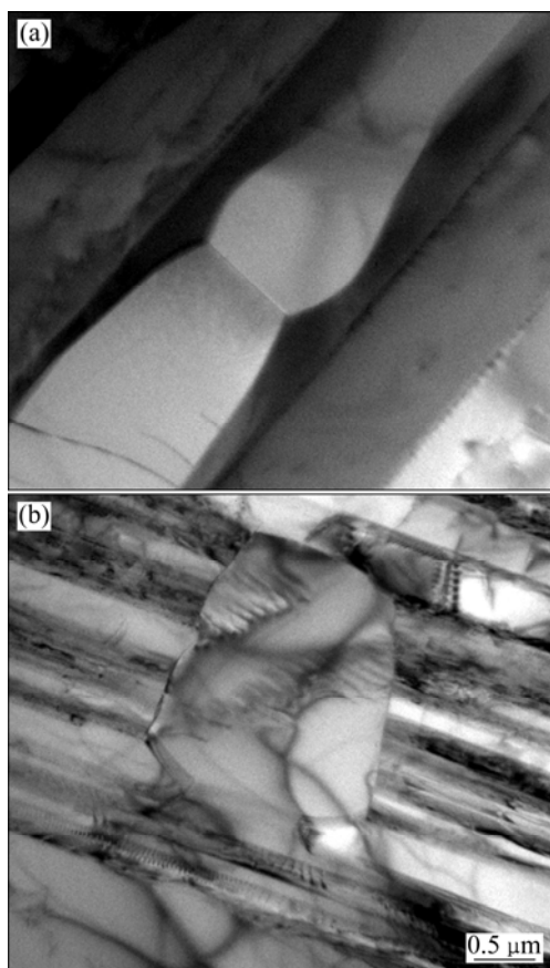
Fig. 8 TEM images of lamellar microstructures after 1000 thermal cycles: (a) Nucleation of \gamma grains in a random direction within \alpha_2 lamellae; (b) Nucleation of \gamma grains in a random direction within ( \alpha_2 + \gamma ) lamellae
