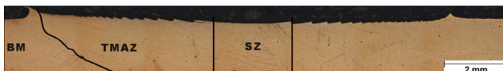
Fig. 3 Cross-sectional view of FSW AZ31 sample
