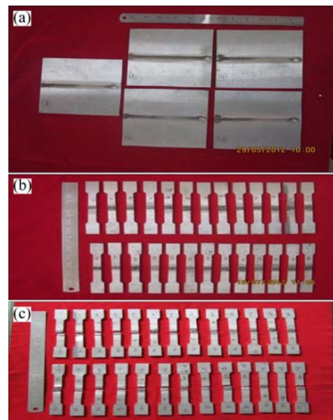
Fig. 2 Photographs of welded joints and tensile specimen: (a) Fabricated joints; (b) Tensile specimens before tensile test; (c) Tensile specimens after tensile test
