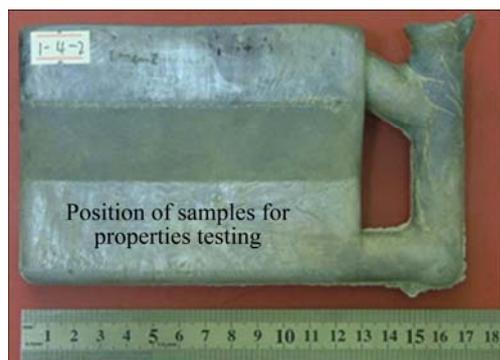
Fig. 1 Casting for mechanical properties tests
