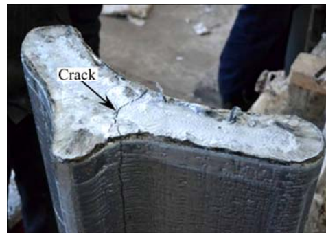
Fig. 15 Casting defects inside ingot
