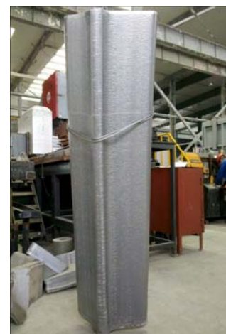
Fig. 16 Near-net shape ingot cast in our laboratory
