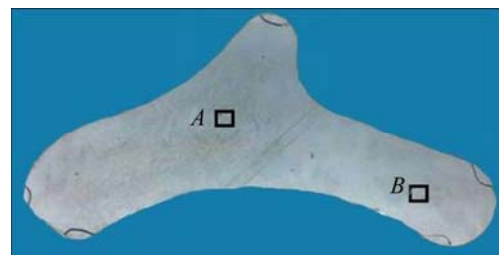
Fig. 11 Embedded points of thermocouples inside ingot
