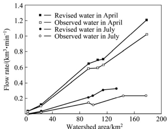
Fig. 4 Water flow rate before and after revision
