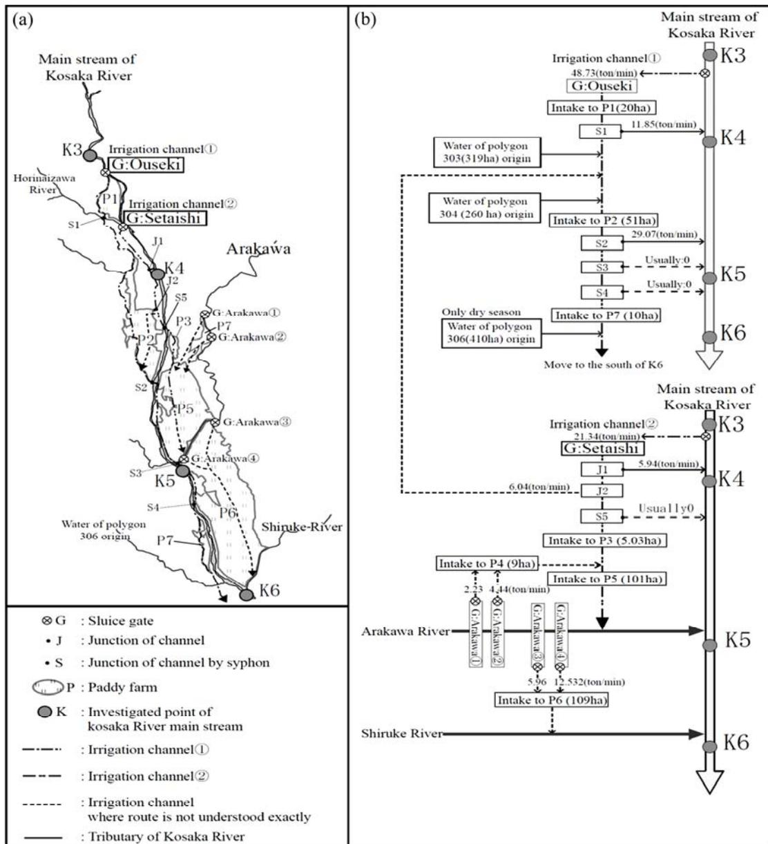
**Fig. 8** Water use route for water intakes and outtakes to main stream: (a) Location; (b) Flow chart (K refers to the P in the text, and K1–K6 respectively refer to P1–P6.)
