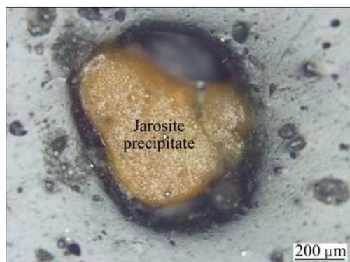
Fig. 9 Polarized light photomicrograph of bio-leaching residue (ferrous sulfate concentration 50 g/L, temperature 32 °C, initial pH 2.2, bio-leaching time 11 d)
