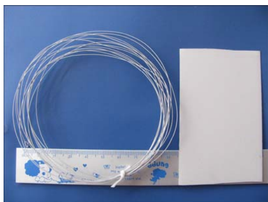
Fig. 1 Optical picture of magnesium alloy wire (left) and sheet (right) after MAO
