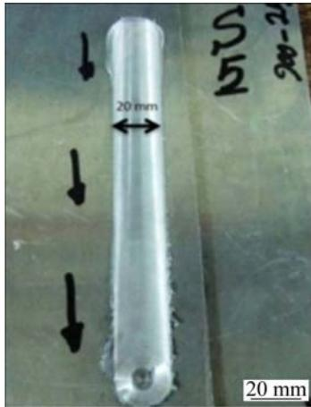
Fig. 3 Sample of friction stir welding in 900 r/min
