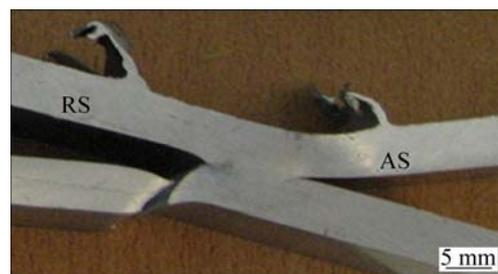
**Fig. 13** Photograph of fracture in lap shear test from retreating side
