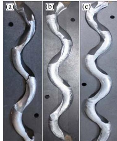
**Fig. 6** Schematic diagram of hanging slurry in serpentine channel: (a) 4 turns, 680 °C; (b) 5 turns, 680 °C; (c) 6 turns, 680 °C
