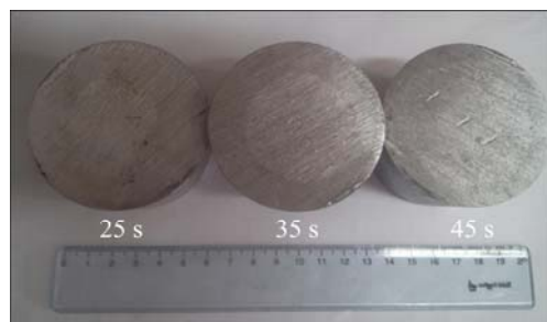
Fig. 2 Macrographs of cross-section of samples produced at 25, 35, 45 s decanting time
